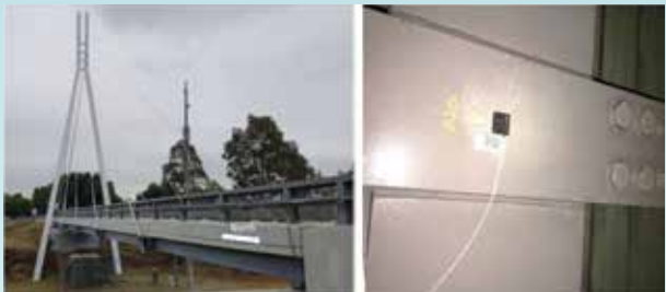
Sensor installation and inspection activities conducted on cable-stayed bridge in Sydney. Fieldwork focused on deploying accelerometers and displacement sensors to collect real-time structural response data
