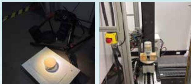
Figure 2. Surface imaging and volumetric scanning of granular soil sample. Left: Photogrammetry setup with controlled lighting and DSLR camera positioned to capture 50 --100 high-resolution macro photos used for 3D surface reconstruction. Right: High-resolution X-ray micro-CT scan of the same cylindrical sample, used to obtain internal structure and reference porosity data for model validation.
