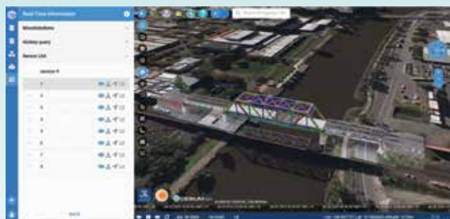
Digital Twin dashboard screenshot showing real-time data and frequency shifts and strain maps for targeted maintenance planning.
