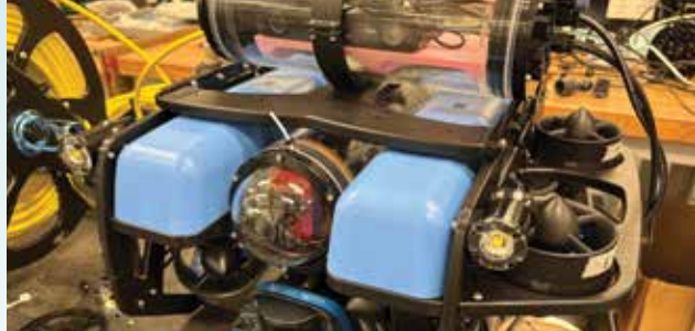
Figure 2. Sensor suite installed on UNSW's existing tethered remotely operated vehicle (ROV)
